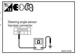
Turn ignition switch ON, and then check voltage steering angle sensor harness connector M47 and ground.
