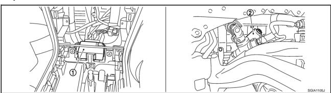
Power steering control unit (Back of center console assembly)
