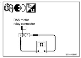
2. When applying or not supplying approximately 12 V between RAS motor relay connector, check continuity RAS motor relay connector B480.
